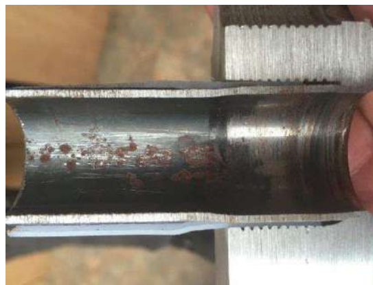
Corrosion of a carbon steel tube.
